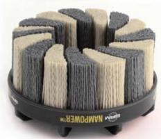
Turbine style disc brushes are ideal for medium and heavy deburring applications. Our unique combination of Silicon Carbide and Ceramic filaments are used to allow the brushes to cut faster and last longer than any other brush on the market. The Turbine style filament is a high density fill that is ideal for short cycle times and long tool life.
